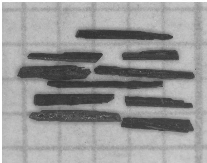
Fig. 1. As-grown needle-shaped \text{NaTi}_2\text{O}_4 single crystals (1 grid = 1 mm).
